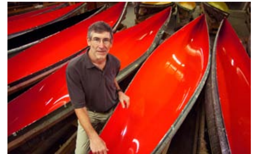
WENONAH CANOE founder Mike Cichanowski displays molds for fiberglass and Kevlar canoes, which may weigh as little as 30 pounds.
